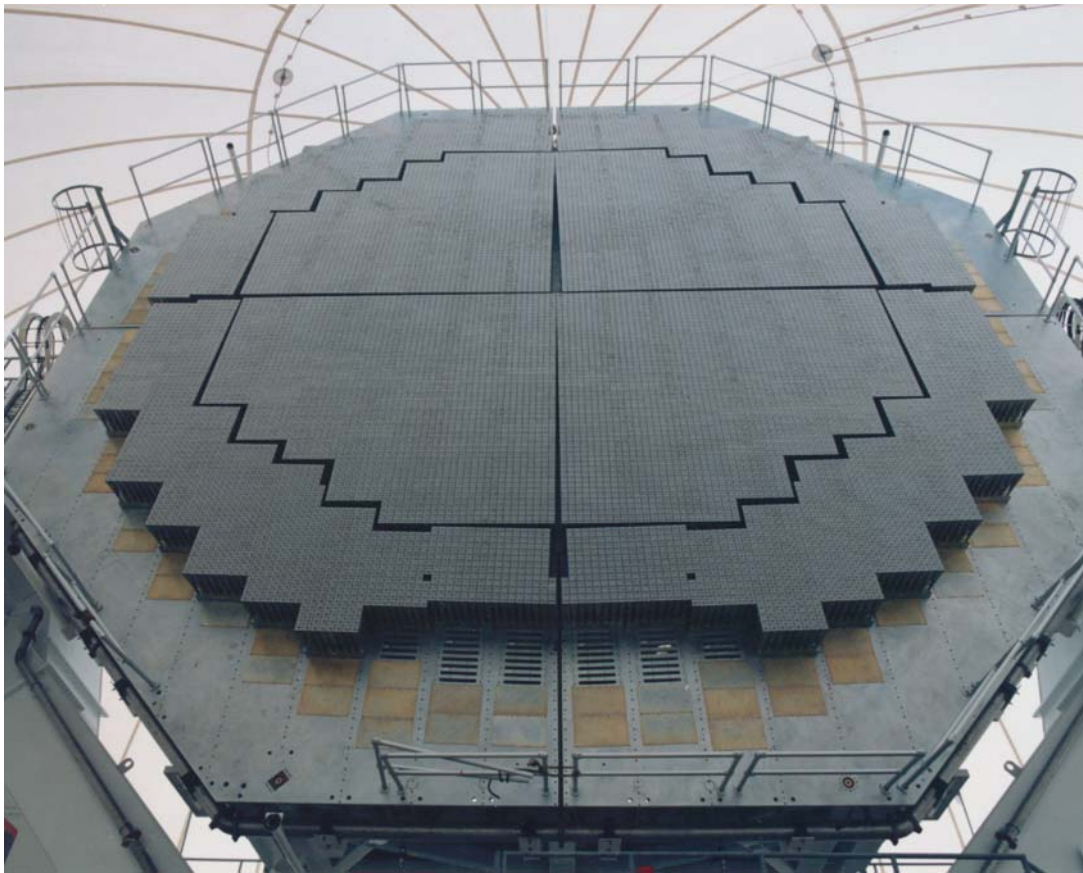
Fig. 6-15. The X-Band Radar can be populated with 69,632 transmit/receive modules. The massive radar stand requires an area of 7 hectares (17.46 acres) for the radar alone.
