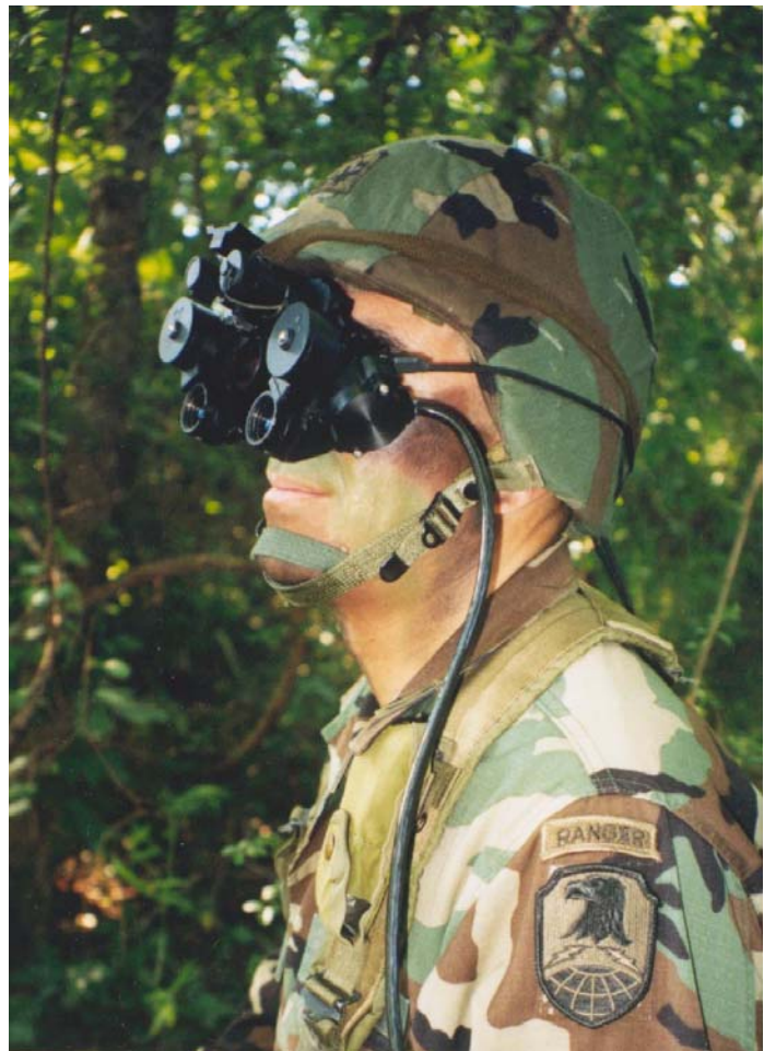
Fig. 6-2. The Uncooled Imaging Technology or UCIT device will enable soldiers to see objects through camouflage, smoke, fog and other
