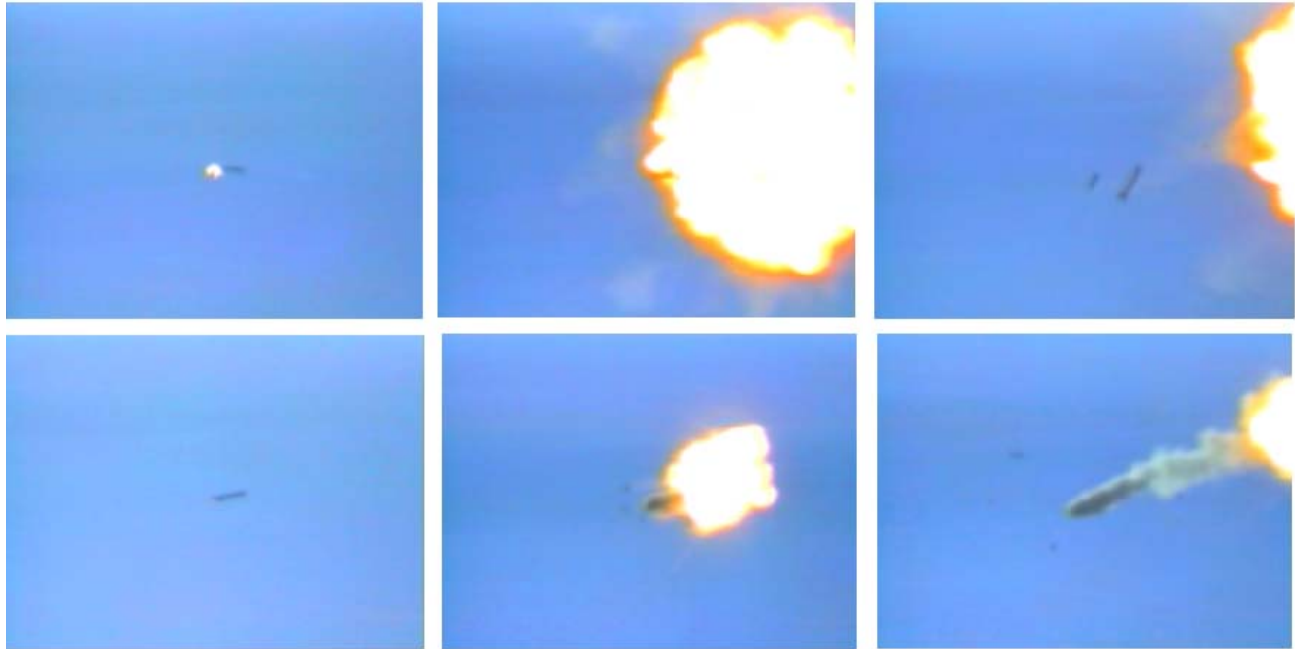
Fig. 6-8. In this series of photos the Tactical High Energy Laser heats the warheads of two missiles to detonate and neutralize them.
