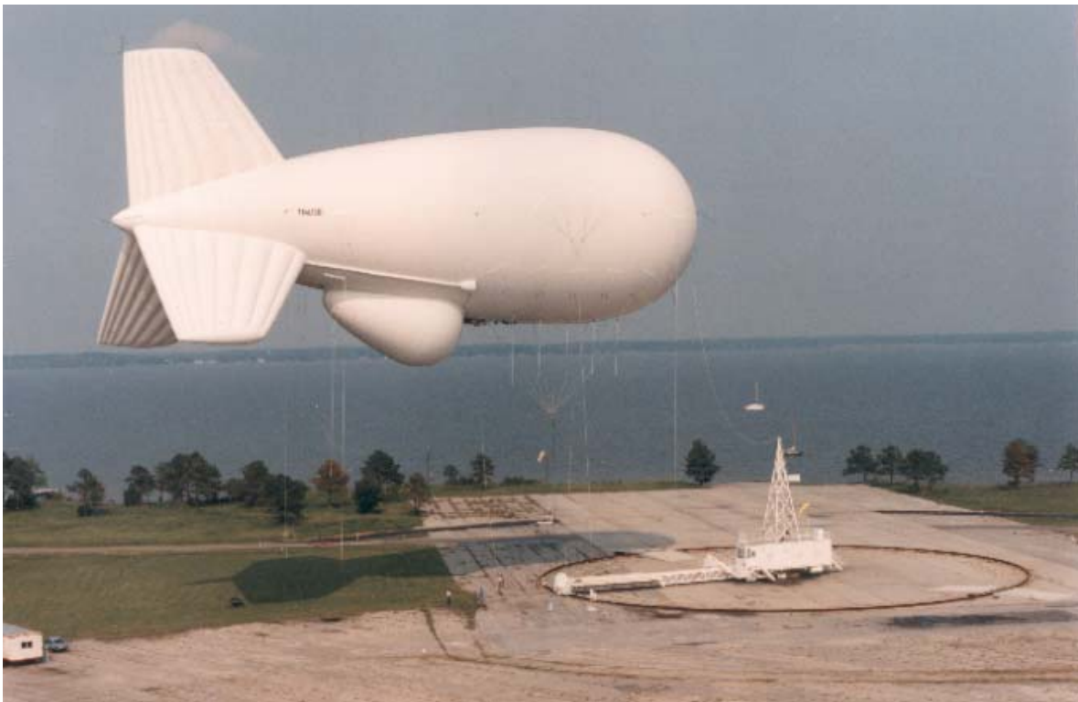
Fig. 6-12. The cost effective Joint Land Attack Cruise Missile Defense Elevated Netted Sensor System employs an aerostat, a tethered helium-filled blimp, outfitted with radar and communications equipment that operates at altitudes between 10,000 and 15,000 feet to see over the horizon.
